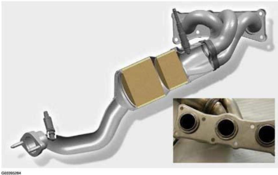
**Fig. 22: Identifying Exhaust Manifold**
