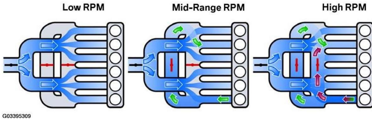
**Fig. 40: Identifying Differential Intake Air Control (DISA) Range Of RPM**
