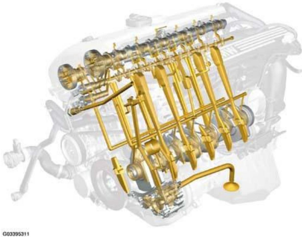
**Fig. 42: Identifying Oil Requirement Components**
