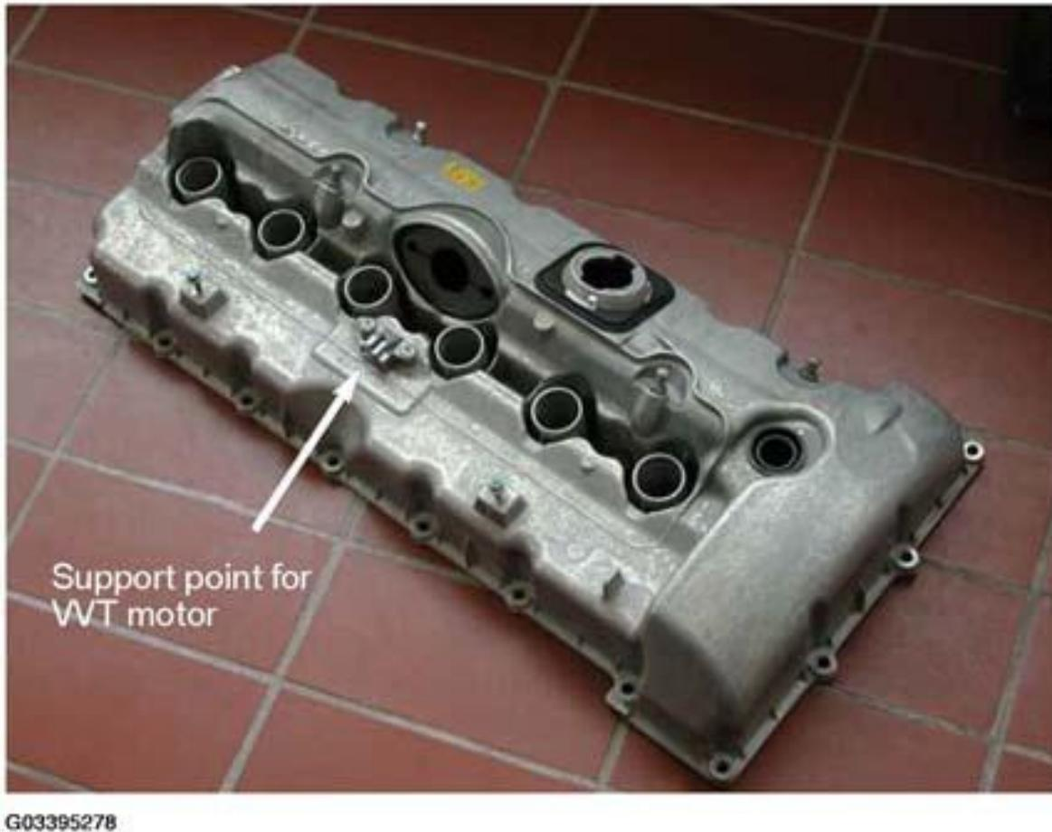
**[Fig. 16: Identifying Cylinder Head Cover](#)**
