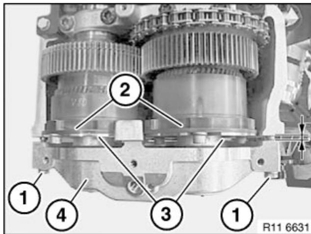
Note: There should be an gap of approximately 8mm at this point during installation.
