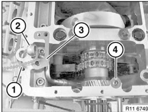
*Re-install VANOS pump, note installation position of the shims (3 and 4 above).*
