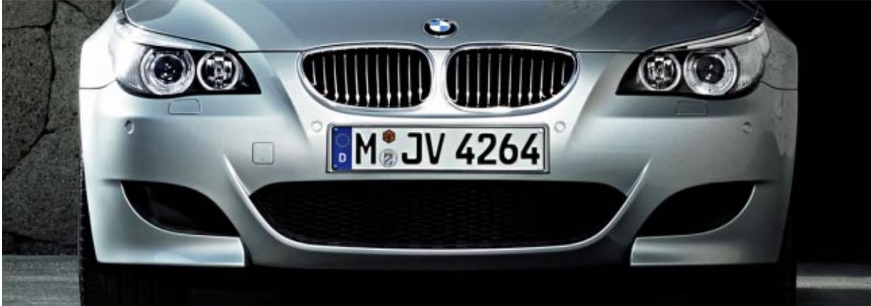
In conjunction with sealing the engine compartment, the front bumper reduces lift on the M5's front axle by 50% in comparison to the standard car.
