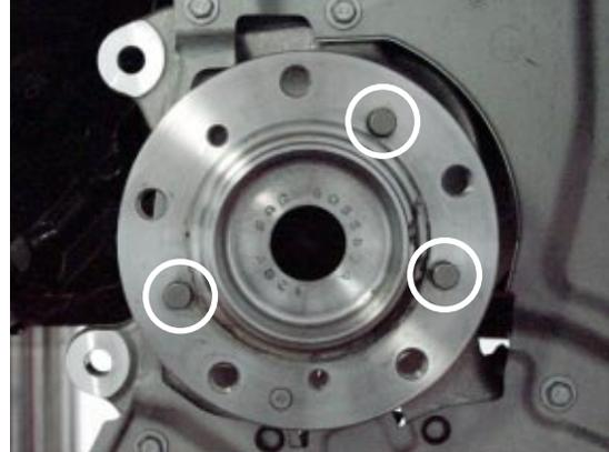
Detail of Rotor Alignment Pins on Hub
