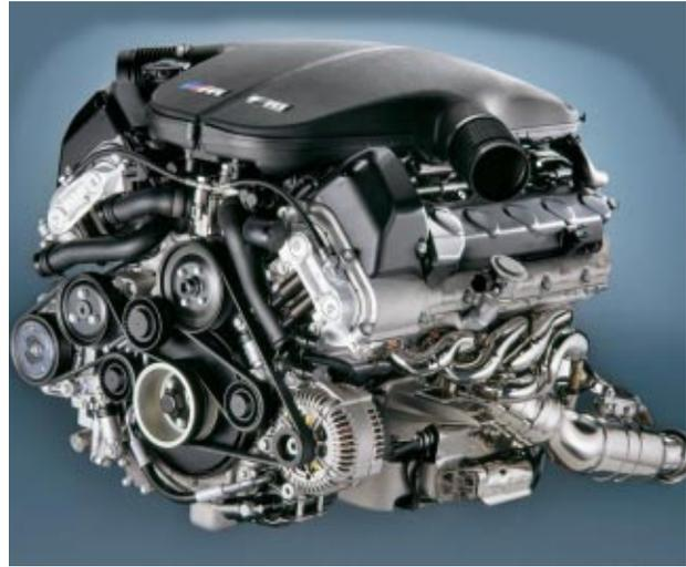
The engine block and cylinder heads are constructed of aluminum alloy and are designed to withstand the demands and stresses of an F1 race. The titanium connecting rods are just one example of components which allow the P84/5 to reach engine speeds of more than 19,000 RPM.
