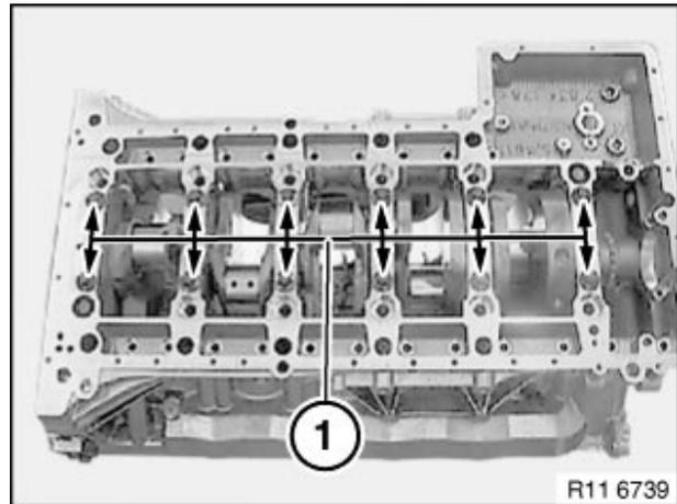
*First remove all M8 fit bolts (#2 - above left) completely from engine. Next, remove the M11 main cap bolts (#1- above right). Then proceed by removing the remainder of the hex (allen) bolts.*
