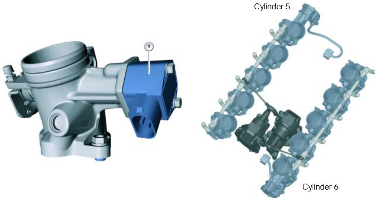
One throttle valve position sensor is located on the throttle housing for cylinder 5 (bank I) and the other is located on the throttle housing for cylinder 6 (bank II). Each sensor contains 2 feedback hall sensors to detect throttle plate position.
