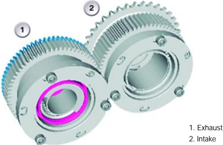
The gear mechanism is driven by the drive gearwheel that interacts with the helical gearing on the inner sleeve. The threaded connections for the gearing connects the inner sleeve to the outer sleeve. With (wide) helical gearing, the inner sleeve acts on the bearing assembly for the drive gearwheel that is firmly secured to the camshaft with the central bolt.
