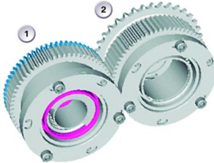
The VANOS transmissions provide the minimum and maximum “spread angle” for the camshafts. The intake camshafts have a spread angle of  $60^\circ$  relative to the crankshaft, and the exhaust camshafts have a spread angle of  $37^\circ$  relative to the crankshaft.
