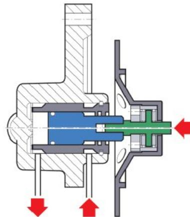
**VANOS Gear Mechanism**
