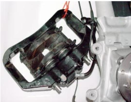
Dual Piston Front Brake Caliper
