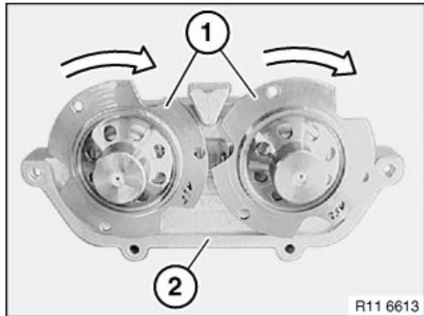
Loosen bolts (see above left picture 1 and 2) 90 degrees. Before installing VANOS adjusting unit, ensure that the thrust plates (see above right - 1) are fully retracted and rotate freely without binding.
