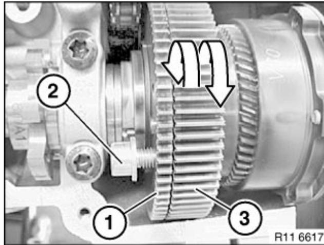
Re-install bolt for timing chain guide rail and install timing chain tensioner. Proceed with installation of the VANOS units.
