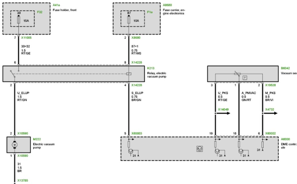
A test module is provided in DIS for the electric vacuum pump. The differential pressure sensor on the brake booster is used for the purpose of monitoring the pump. The plausibility is checked by the pressure difference between the vacuum and ambient pressure calculated internally in the ECM. It is evaluated and, in the case of fault, shown in the instrument cluster and displayed as a CC message (check control).
