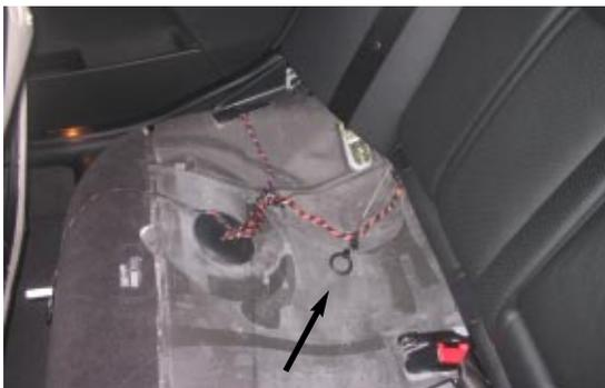
**Mechanical Release for Trunk**
