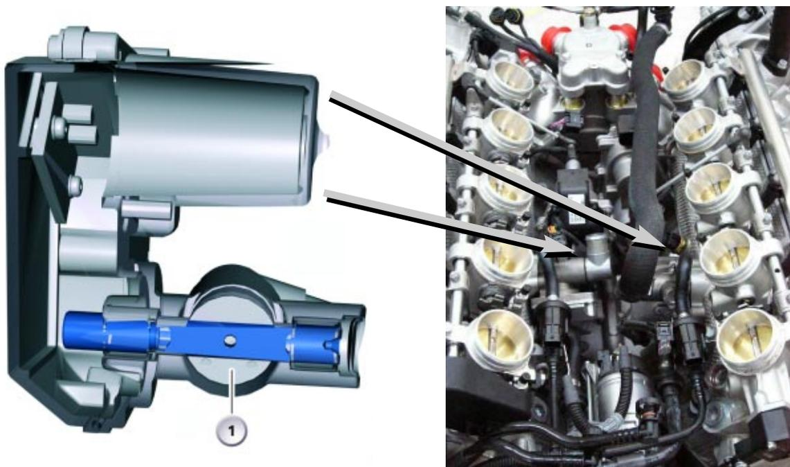
The engine control module determines the current actual load signal from the throttle valve sensors (DKG) and feedback signals from the LLS actuators in order to check the setting of the throttle valves. The plausibility of the load signal is checked against the signals of the two hot-film air mass meters.
