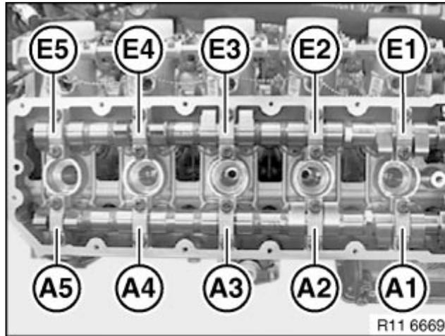
Depress camshafts with special tool and secure bearing caps. Do not tighten the camshaft bearing caps to full specification on the trainer engine.
