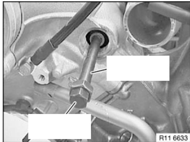
Install M8 X18mm lock bolt (2) on the exhaust VANOS gear as shown below. Tighten fully to prevent slippage of split gear mechanism (1 and 3).
