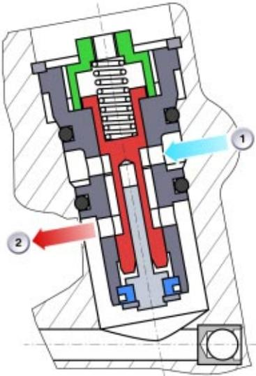
The high pressure pump consists of the fixed stator about which the rotor rotates. Five moving plungers are mounted in the rotor. The stator and rotor are installed off-center in the pump housing. The plungers are guided radially as the rotor rotates thus producing the pump stroke motion.
