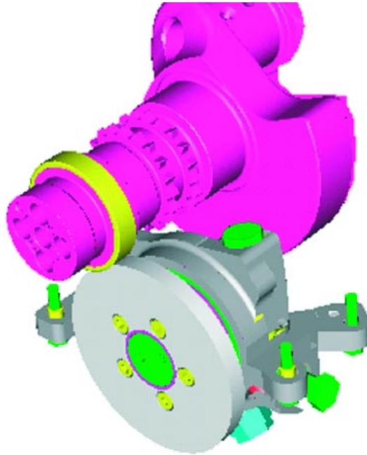
The high pressure pump receives its oil supply from the bedplate. An 80 micron fine filter is installed in the transition hole from the bedplate to the high pressure pump. This filter has the sole purpose of holding back any impurities that may accumulate during series production and is not replaced during vehicle operation.
