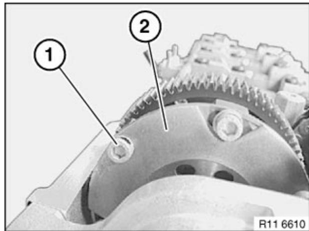
*Remove 6 bolts (reference #1 on graphic) on each VANOS adjusting unit, rotate engine to access all bolts on both banks. Proceed with removal of both VANOS adjusting units as per repair instructions.*
