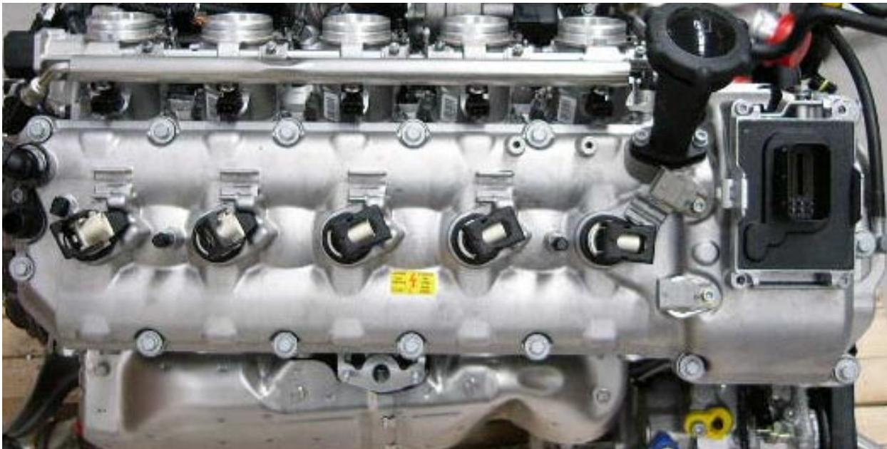
*Re-install cylinder head covers, ignition coils and the ionic current control units.*
