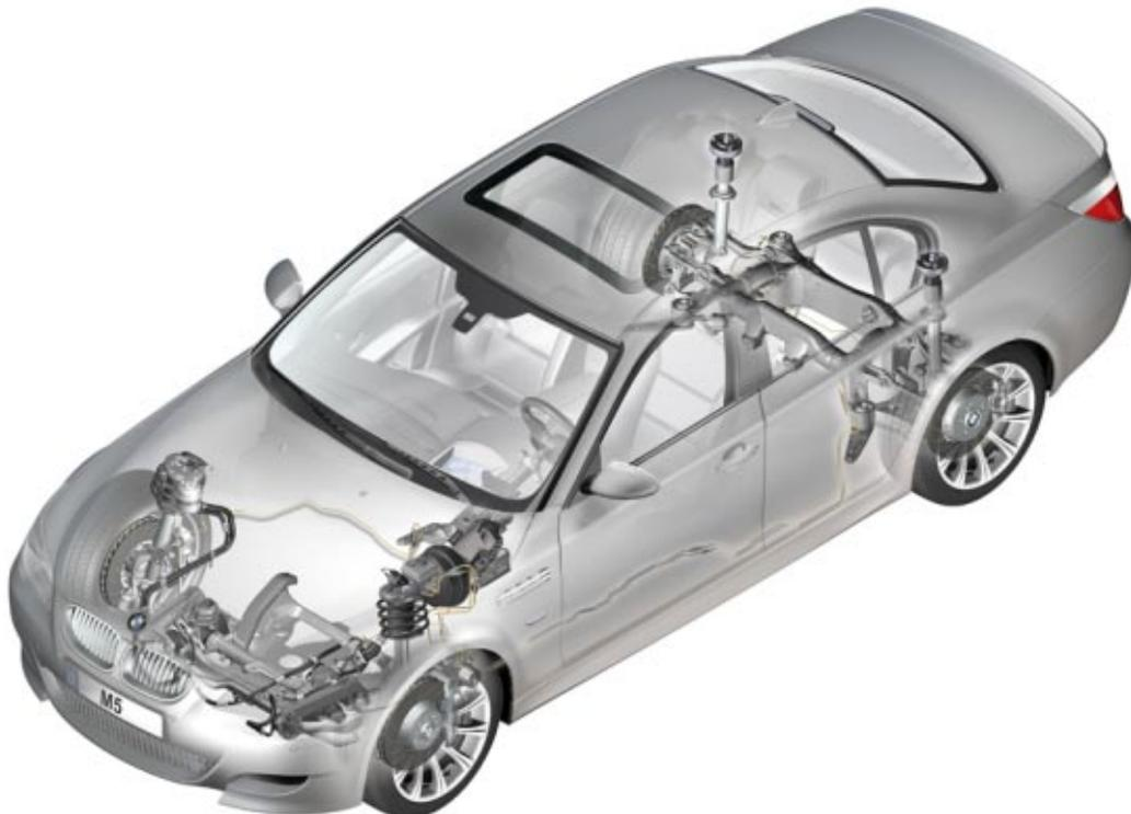
The suspension system used on the E60 M5 is carried over from the production based E60 5Series sedans.
