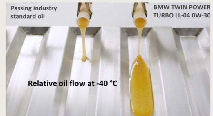
(1) Based on NOACK volatility test; (2) BMW Specific Fuel Economy Testing expected in 2016; (3) Compared with higher viscosity oils tested using ASTM D5293
