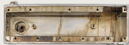
Images show industry standard valve covers comparing the use of BMW Longlife-01 SAE 5W-30 with that of an inferior, SN capable, oil.
