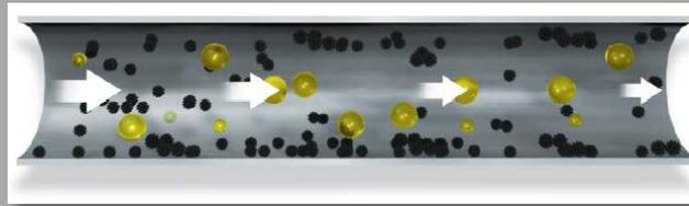
Sludge build-up is caused by combustion by-products that stick together.
