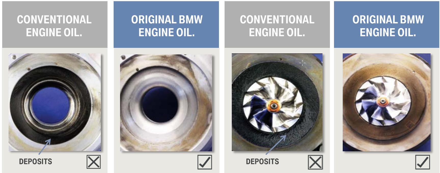
Images show compressor back plate and housing. Tests have been conducted on a turbocharged BMW N47 under high temperature operation.
