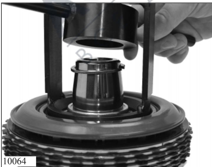
Press down the support disk with the pressure pad 5x46 000 167 under the mandrel press and secure it with a new snap ring 75.220.
