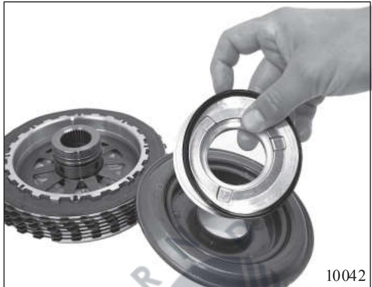
Remove the disc spring and multidisc package.
