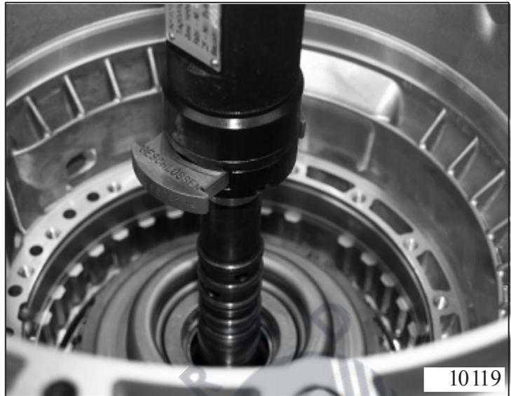
Insert brake B beginning with end disk 72.040, then alternately lined disk 72.030 and outer clutch disk 72.020, and finally spring clutch disk 72.010.
