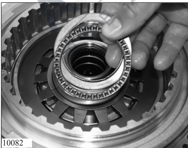
Fit an angle disc 70.100 and needle bearing 70.090 in the oil supply (cylinder A).
