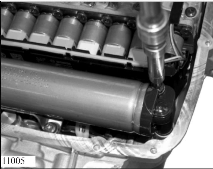
Unscrew 3 torx screws from oil volume accu.
