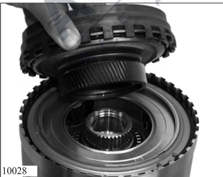
Remove internal ring gear 2 with sun gear 3 from pot 2.
