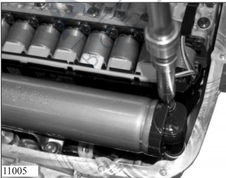
Fit a new O-ring in pressure socket from
