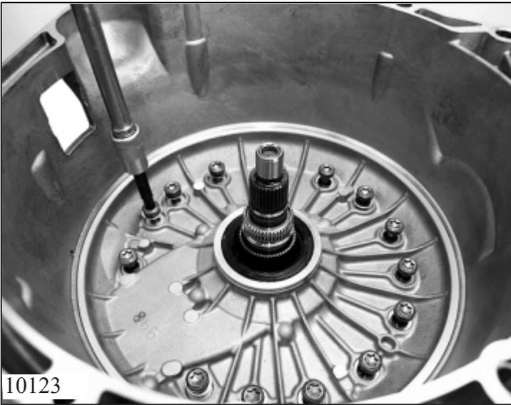
Secure the oil supply with 14 new screws 10.230.
