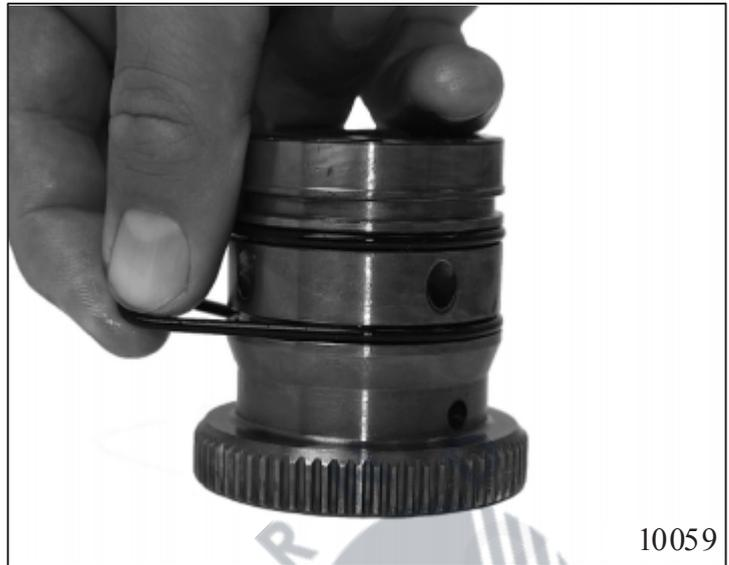
Fit the hub into cylinder C 75.050.
