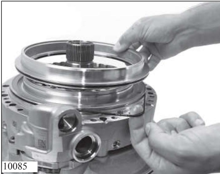
Mount new O-ring 72.140 onto intermediate plate.
