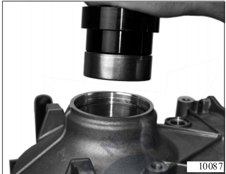
Position a new sealing sleeve 14.030 onto tool 5x54 909 281 and mount into the transmission housing.
