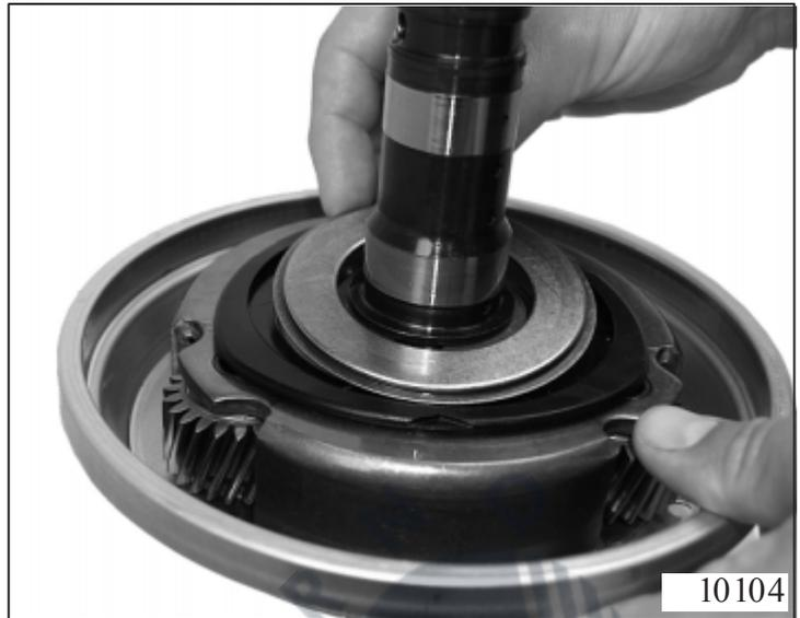
Insert input shaft into tower.
