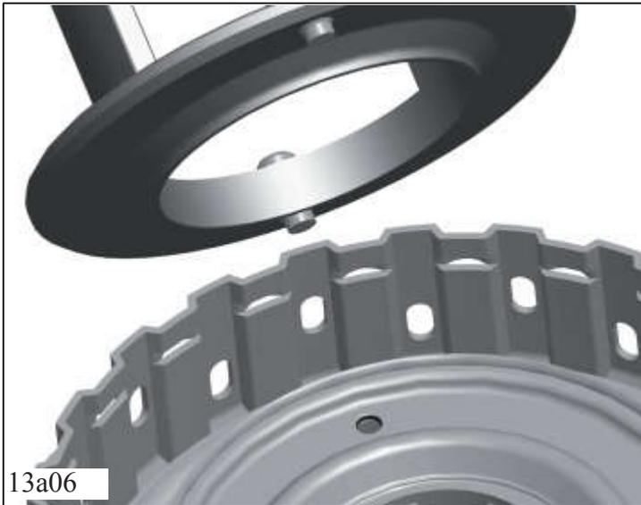
Position tool AA00 349 340 with both pins in baffle plate.
