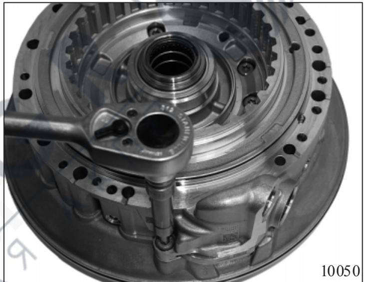
Remove the O-ring from the intermediate plate.
