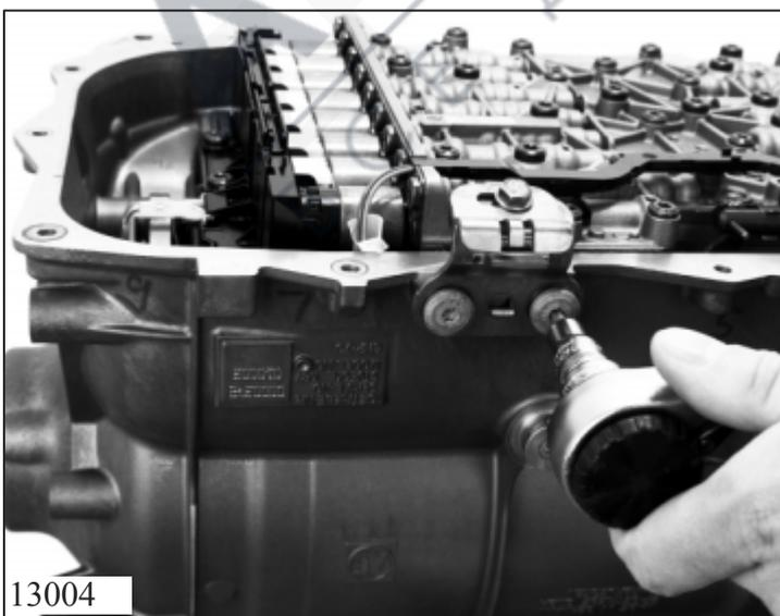
Unscrew 2 screws from the holder (emergency release puller) and remove the holder.
