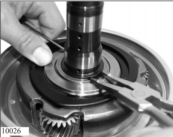
Leverage out thrust washer from planet carrier 2.
