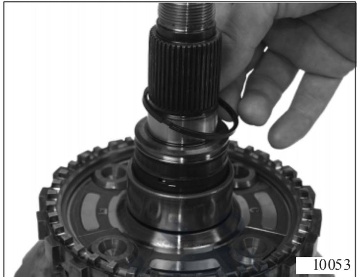
Insert the output shaft in the mounting device.
