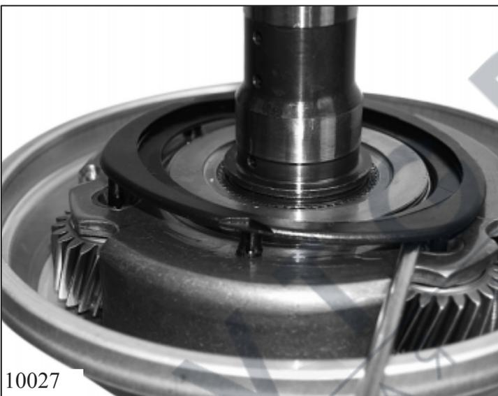
Leverage out oil tray from planet carrier 2 with screwdriver.
