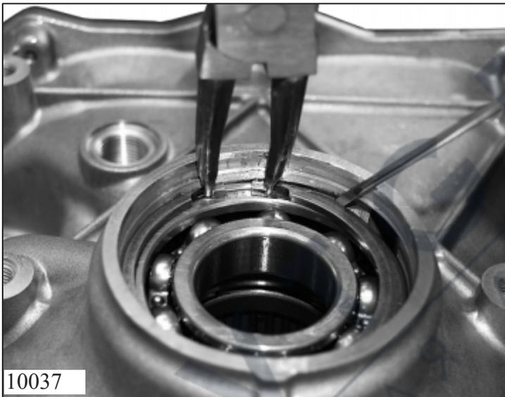
Remove the snap ring from the ball bearing.
