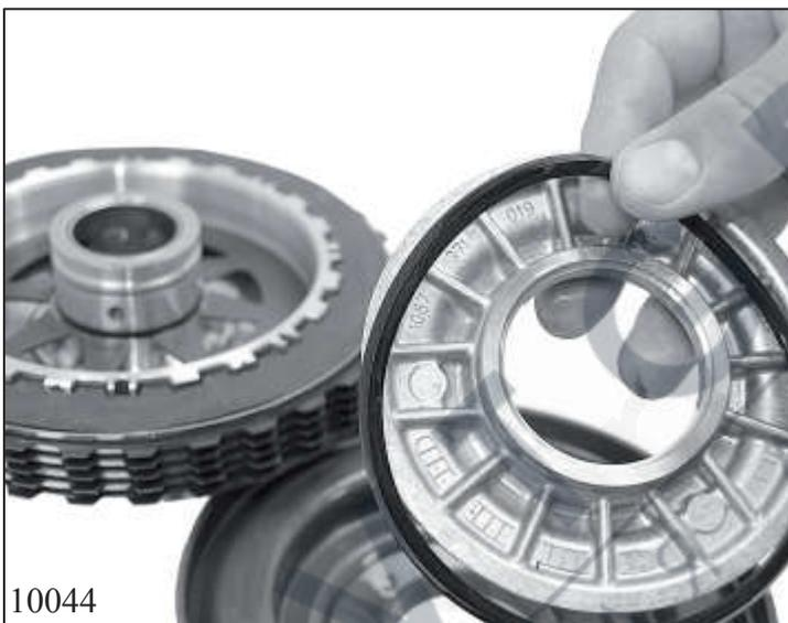
Press down on to the baffle plate using pressure pad 5x46 000 167 and remove the round wire ring.
