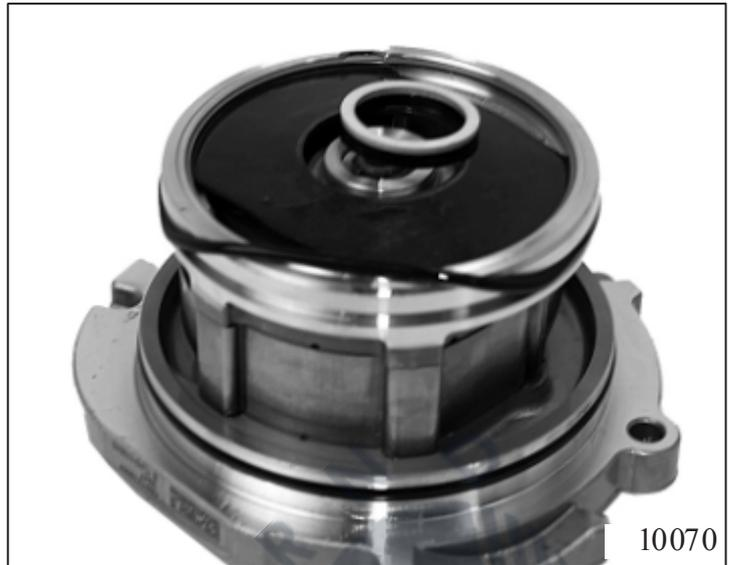
Fit the pump with chain 10.060 and drive sprocket 10.080 on the intermediate plate 10.010.
