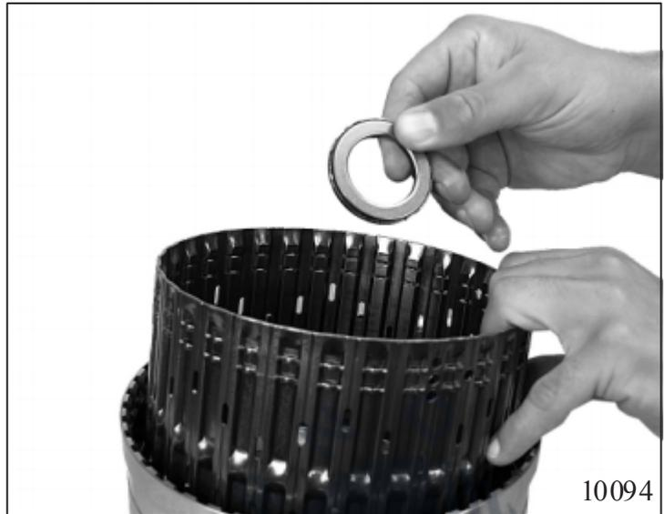
Insert clutch C into sun shaft.
