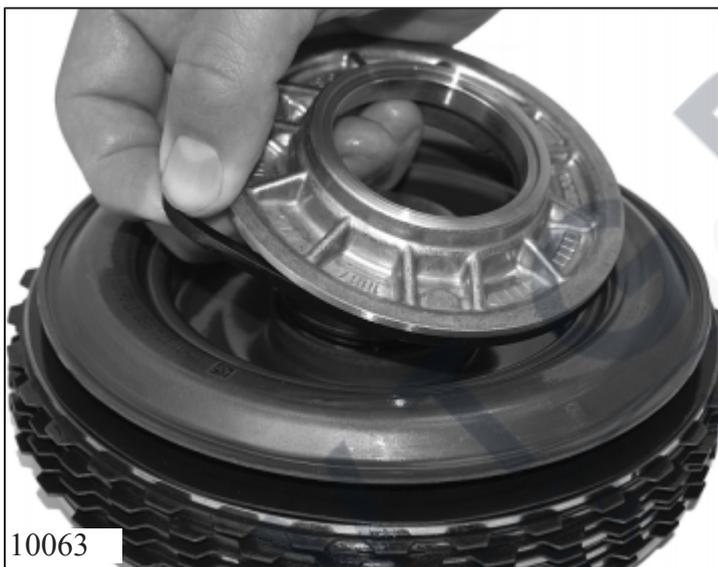
Press support plate 75.180 with a new lippered seal ring 75.200 into piston C.
