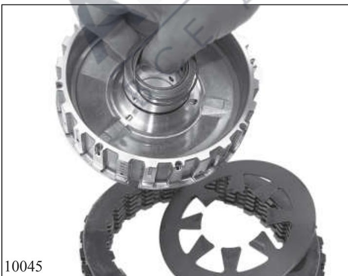
Remove the disc spring and multidisc package.
