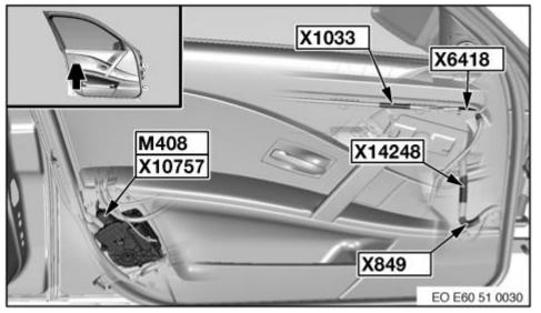
Fit the driver's door mirror and fit the rubber grommet, remember to put the foam padding back as well, screw in the three torx bolts and connect the new connector.
