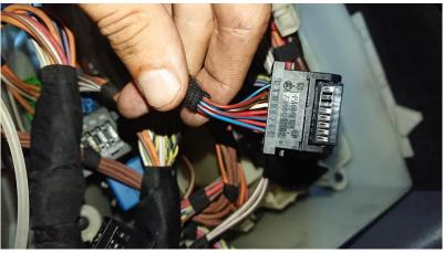
Before pinning the connector with the new wires, there is a pin holder that must be carefully raised from the sides in order to allow pins to settle in their sockets. Once done, you should end up with something like the following picture:
